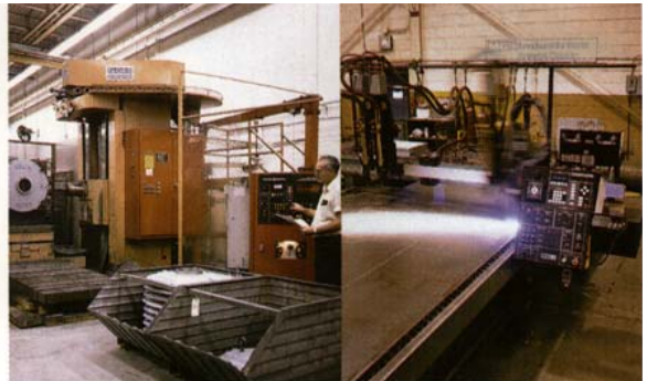
This computer-controlled machining center (left) and computerized cutting table (right) typify the advanced precision methods used in manufacturing ROTEX
