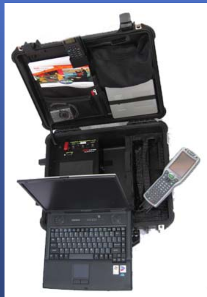
Long life NiMH Batteries 100-240Vac power 10-32Vdc power
